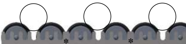
SPACING FOR 20 ROLLERS (10 PAIRS) – NOTE THE EXTRA-WIDE SPACES *
