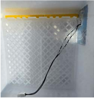
The supplied plastic hatching mat didn't cover the work screw through which could be a hazard to hatched chicks
