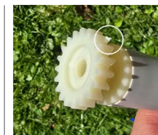
Minor faults on the gears can lead to them jumping out of the worm screw
