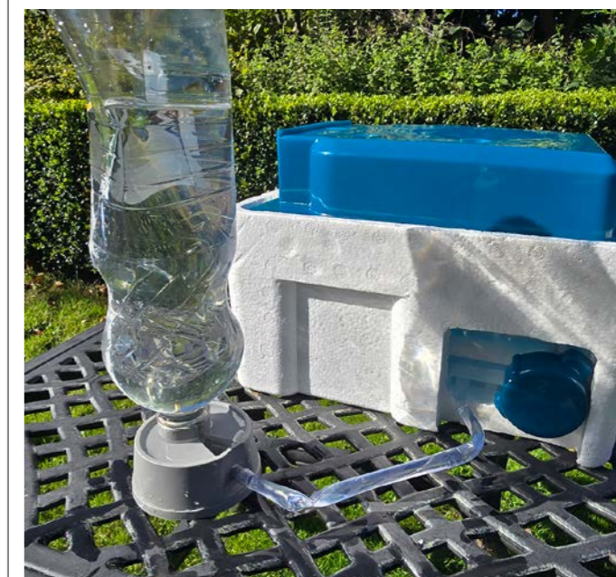
A pipe and pod for a water bottle allow water to be added via a gravity feed into the incubator
