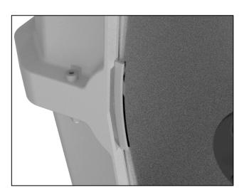
Open the door wide and press the door edge strip into place on the door. Close the door and check the strip does not force the door outward. Trim the length of the edge strip if necessary.
