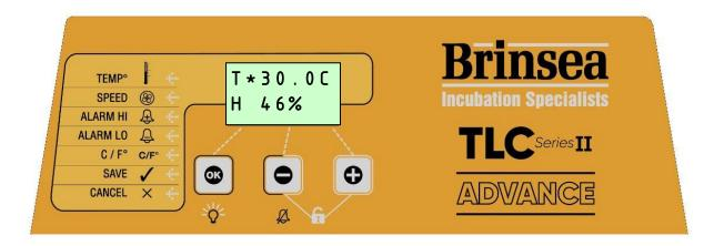
The TLC Advance Series II control system utilises highly accurate, individually calibrated sensors for temperature and humidity. Be cautious of low-cost analogue or digital thermometers and hygrometers when comparing them with the brooder/ICU display readings.
