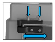
Loosen the top hinge/cabinet fixing. Move it so that the door becomes level in the frame and opens/closes freely. Tighten the fixings.
