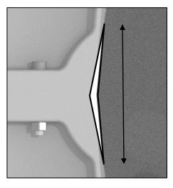
Observe the length of any 'V' shape gap that a claw could fit through. Cut the door edge strip to fill the length of the gap.
