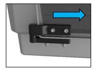
Slide the door as far as it will go in the direction of the door latch. Tighten the fixings while holding the door.
