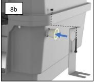
4.5 If caring for small animals with long claws such as hedgehogs, the door edge strip may be fitted as shown to ensure claws cannot pass through any door gap:
