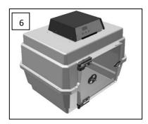
Fit the M4 x 30mm cap-headed screws, star washers and nuts into each set of holes around the edge of the cabinet. Tighten enough to prevent them spinning. This creates an air tight seal around the cabinet. If the nebuliser is required, fit the nebuliser bracket as shown (8a). If the nebuliser is not required fit the grommet first and secure it with the bracket (8b).
