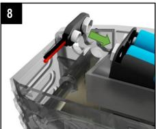
Fit the connector to the battery holder.
