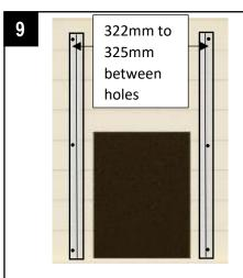
Once the channels are vertical and the holes are 322mm – 325mm apart, mark the locations for the six fixings. Drill 1.5mm diameter holes.
