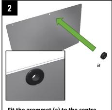
Fit the grommet (a) to the centre hole in one door panel.
