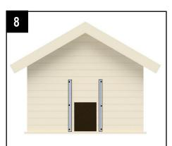
Position the channels on each side of the door hole on the hen house with the hole central between the channels. They must be perfectly vertical, flat and level. The fixing holes must be 322mm – 325mm apart.
