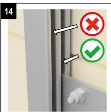
It must be in the second slot in each channel. The screws and nuts must be at the front.
