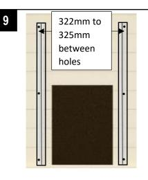
Once the channels are vertical and the holes are 322mm – 325mm apart, mark the locations for the six fixings. Drill 1.5mm diameter holes.
