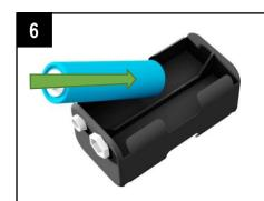
Fit the 4 batteries into the holder.
