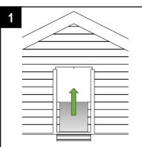
Raise the sliding door to its fully open position.
