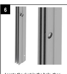
Locate the rivet in the hole, then push it in to secure it.
