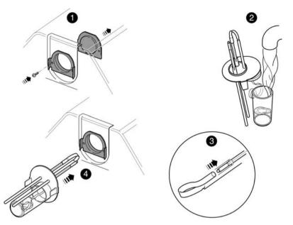
You will need a piece of stiff wire about 8cm long (e.g. paper clip extended straight), a phillips screwdriver and a small amount of distilled water.
